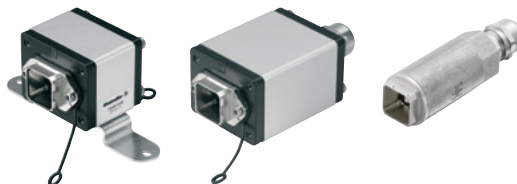
FreeCon: junction box/coupling and cable coupler for PushPull signal or PushPull data connectors. Installation options: at the front on a mounting plate or with supplemental mounting foot. Installation of the cable coupler: flying or with additional support frame
