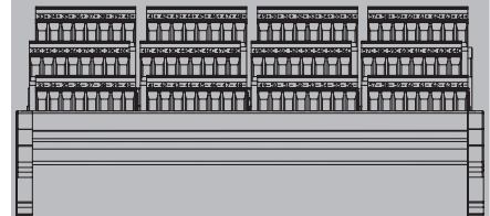
Field terminals view for ADV161 (Channels 33 to 64)
