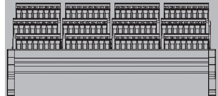
Field terminals view for ADV161 (Channels 33 to 64)
