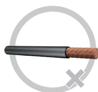
Excessively twisted individual wires
