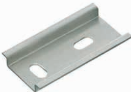
TS 35/7.5 mm according to EN 60715 (s = 1.0 mm)
