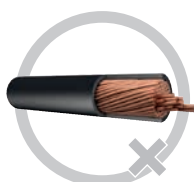
Pulled out conductor
