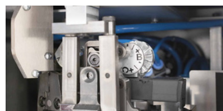
Adjustable trigger sensor for optimum stripping length
