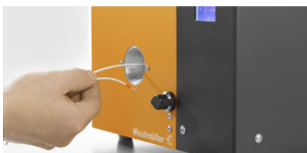
Stripping and crimping in one step
