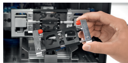
Quick-change tool for extremely short retooling times
