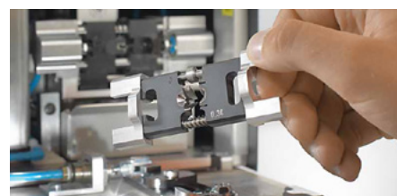
Quick-change tool for extremely short retooling times
