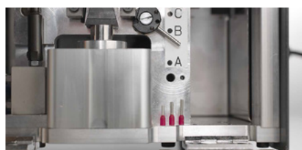
CRIMPFIX LS: three different crimping lengths – no need to change tools
