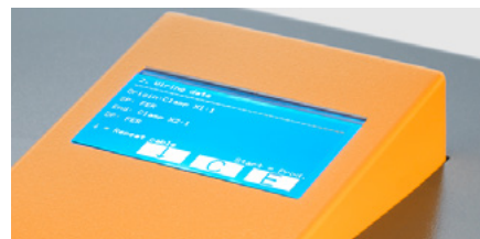
Read out of the wiring data on the display
