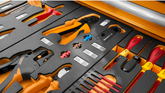
If a tool is missing, the recesses and MultiCard markers make it easy to identify
