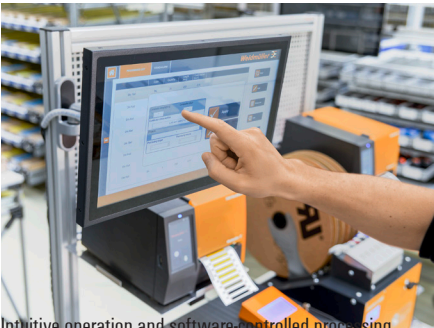
Intuitive operation and software-controlled processing via the touchscreen
